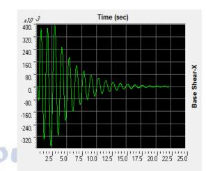
Fig 10:- Base Shear-Time history of building with isolator
