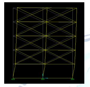
Fig3 :- Deformed shape of fixed base model
