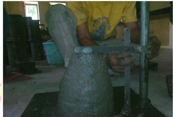
Fig 1 Slump of concrete being measured in Laboratory
