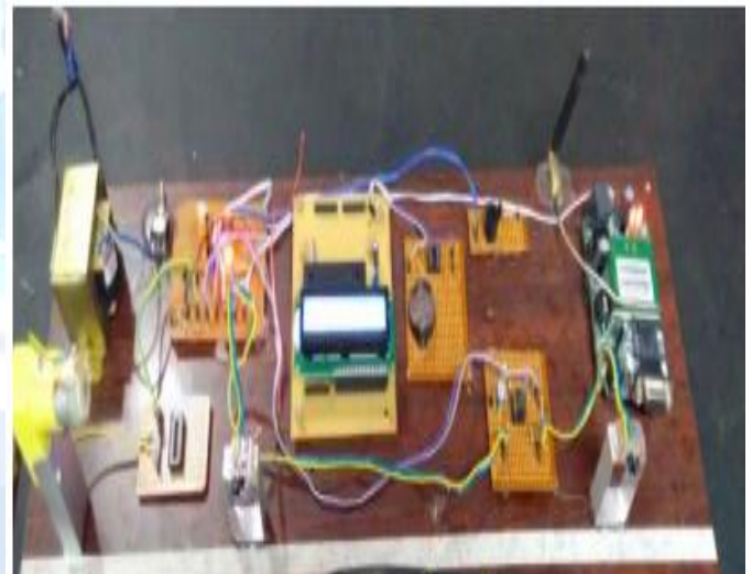
Figure 3: Automatic Toll Collection System using RFID & GSM Technology
