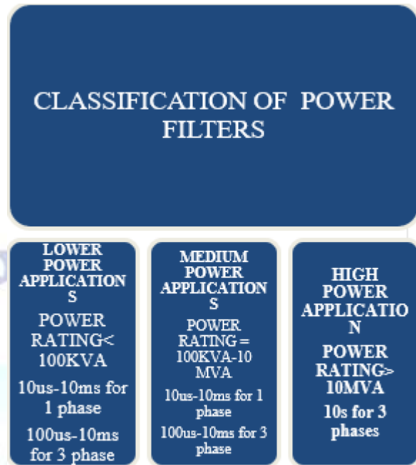
Figure 1 illustrates the segmentation of power filters based on their power rating and response speed.
