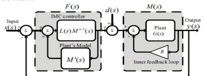
Fig (2): The 2DF IMC configured as a PI controller
