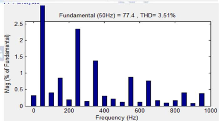
Fig.8: % THD of supply current (a) before compensation (b) after compensation.
