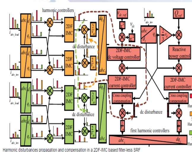
Fig (4): Harmonic disturbances propagation and compensation in a 2DF-IMC based filter-less SRF
