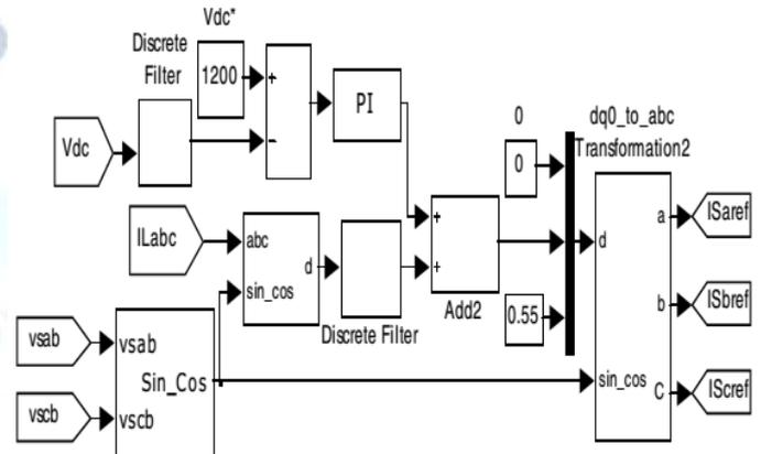
Fig (5) Conventional SRF-PI model in matlab/simulink
