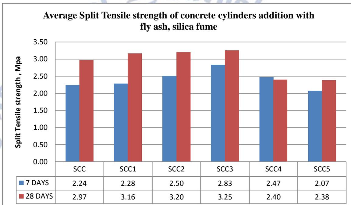
**Average Split Tensile of concrete cylinders addition with fly ash, silica fume And fibres**
