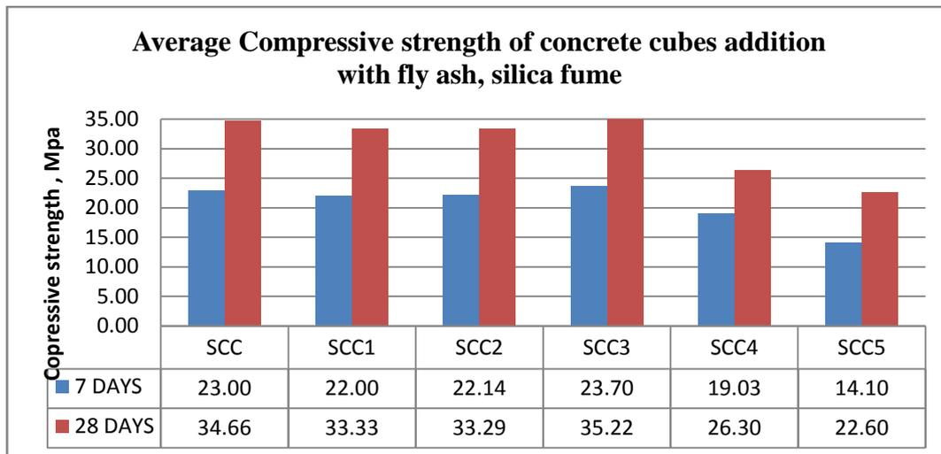
**Average Compressive strength of concrete cubes addition with fly ash, silica fume And fibres**
