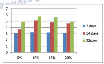
X-axis:-'%' of replacement Y-axis:-flexural strength
