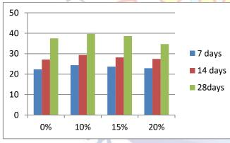
X-axis:-'%' of replacement Y-axis:-compressive strength
