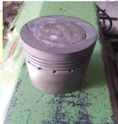
Fig: 1. Filling with welding Aluminum metal
