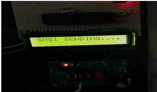
Fig 5 After detecting the block, the message is sent to the higher authority in municipality.
