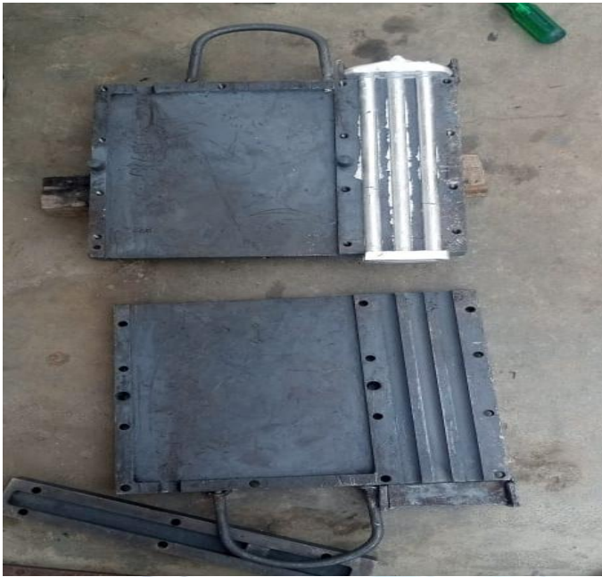
Figure 2: Aluminum with rice husk ash particles composite material with 8%,12%,15% RSH particle rods.
