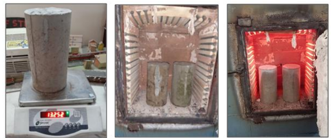
Fig. 6.7 Specimens Before Exposure and After Exposure
