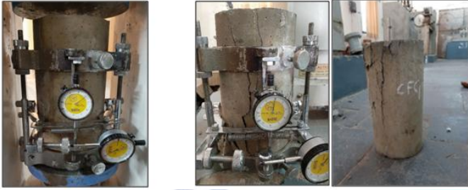
Fig. 7.2.1. d. Cracks of Concrete Cylinders
