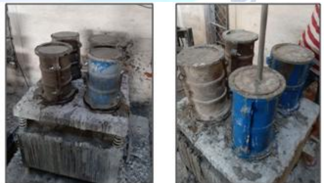
Fig. 6.5 Compaction of Concrete
