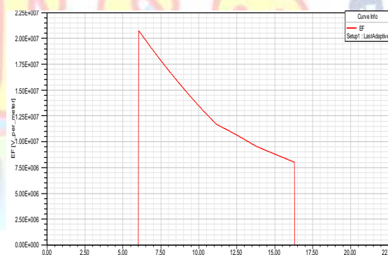
Fig 9: Electric field distribution in cable without defect
