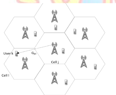
Fig.1. G_{jkl} is channel matrix between user k in base station l and M antennas in base station j.
