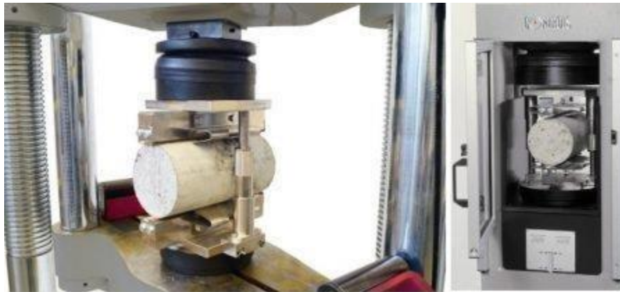
testing cylinder on compression testing machine
