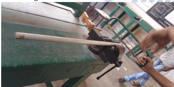
Fig 2: Cutting Aluminum rod into pieces
