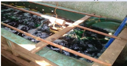
Figure 7 Electrochemical coating on cutting tools
