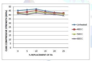
Compressive strength of cubes when exposed to  $400^{\circ}$ C,  $500^{\circ}$ C,  $600^{\circ}$ C at 28days for 60 minutes duration
