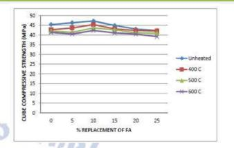
Variations in compressive strengths at 28 days duration exposed to  $400^{\circ}$ ,  $500^{\circ}$  &  $600^{\circ}$  C for 60 minutes duration.
