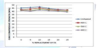
Variations in compressive strengths at 400  $^{\circ}$  C, 500  $^{\circ}$  C, 600  $^{\circ}$  C at 56 days duration for 30 minutes
