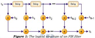
The process of selecting the filter's length and coefficients is called filter design. The goal is to set those parameters such that certain desired stop band and pass band parameters will result from running the filter.
