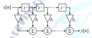
Figure:2 Basic Structure of an FIR Filter
