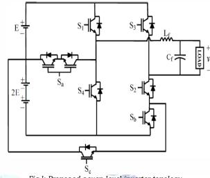
Fig.1: Proposed seven level inverter topology.
