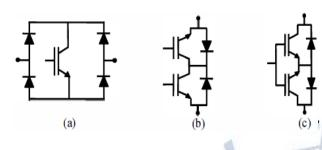
Fig. 2 Bidirectional switch configurations
