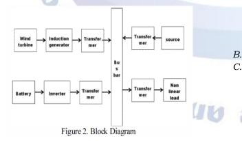
Figure 2 represents the block diagram of static compensator with non linear load. Normally induction generator IS used in wind energy generating units.
