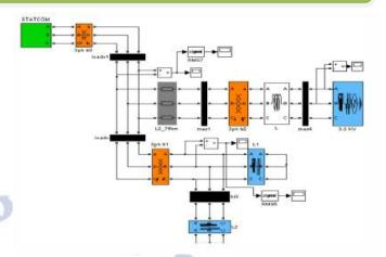
Figure 6. Circuit diagram with STATCOM model
