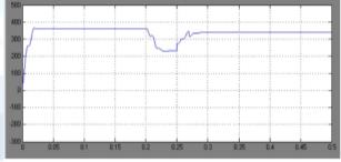
Figure 9.RMS Load voltage with sag conditions
