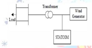
Figure 1. Voltage Fluctuation Mitigation with STATCOM
