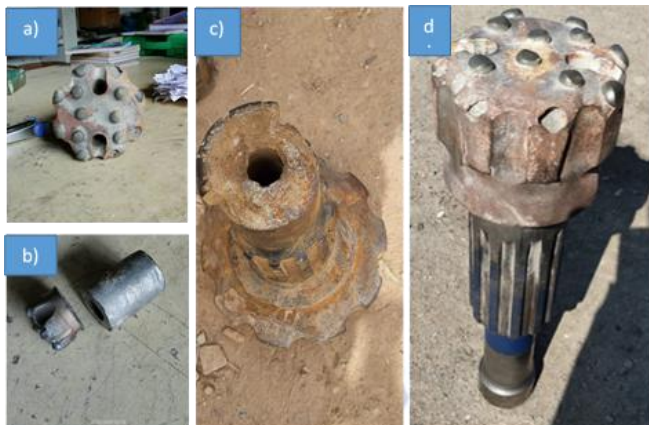
Fig-1 Various Failure modes of drill bits
