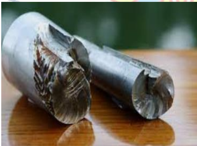
Drive shaft failure while it is still operating
