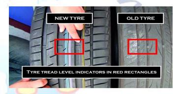
By looking at the level of the rubber, we can determine the tyre threading. Every tyre will have one, and it will allow you to see when the threading on the tyre has worn out. If the thread size is correctly read, we may either change the tyre or recall that it was worn out and proceed with caution when driving.
